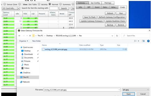
c. Reboot the FlexControl Module or Card. NOTE: The actual installation of SncLog addon firmware occurs on the reboot of the system after code upload!
